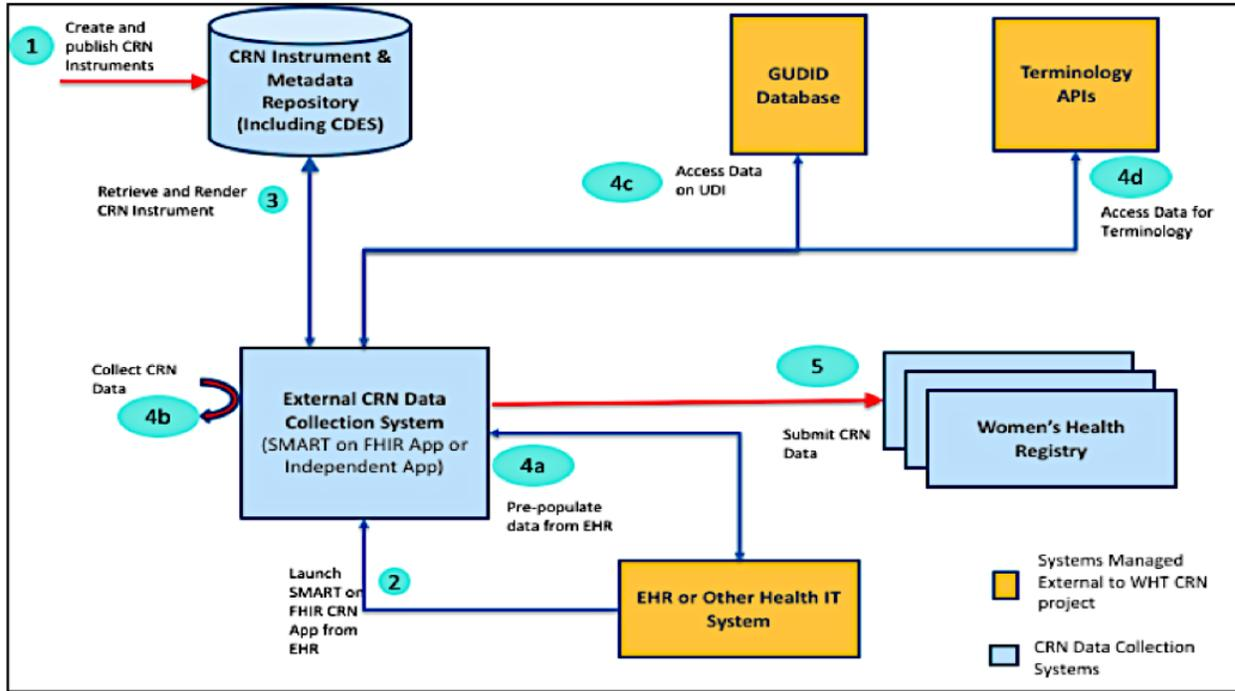
**Figure 13: The abstract model, actors and the data flow to access collected data from registries**
