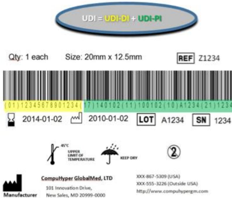
UDI comprises of UDI-DI (UDI-Device Identifier and UDI-PI (UDI- Production Identifier). The UDI must be present on the label of a device in machine readable and human readable formats
